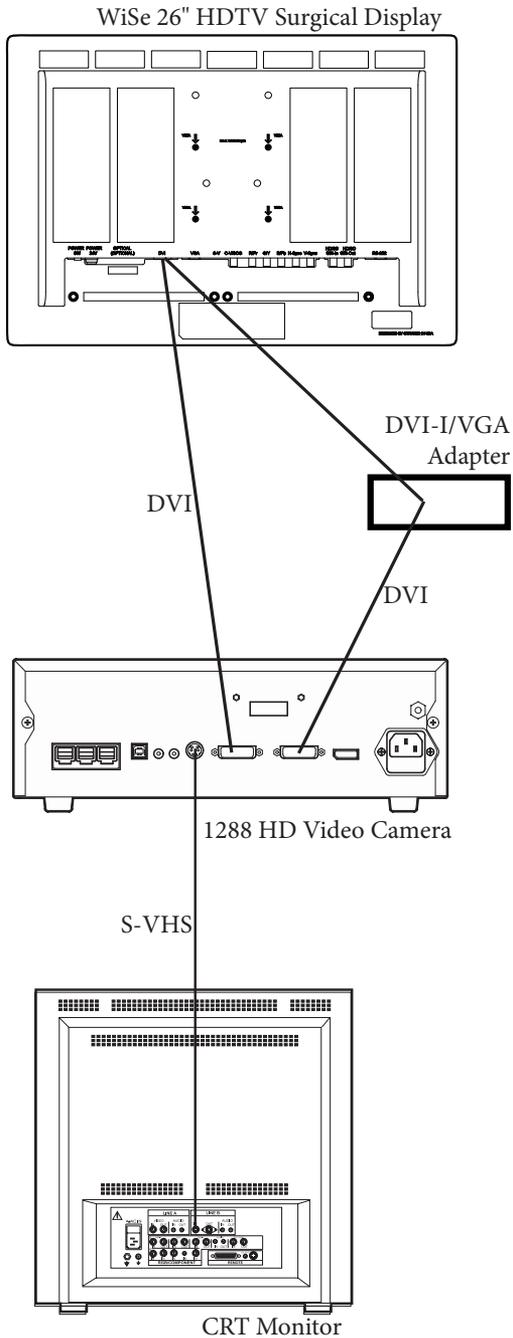
**Note:** If you are using any device with unterminated analog video inputs, you must connect a cable from the VIDEO OUT of that device to the VIDEO IN on the monitor.
