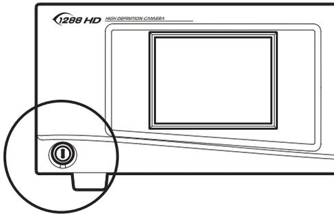
Press the power switch on the console to power the camera on or off.
